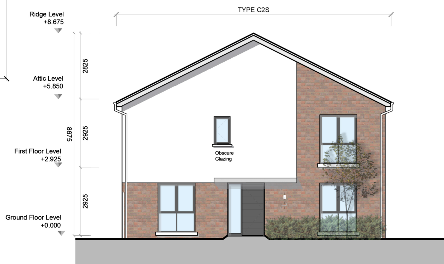
SIDE ELEVATION (SIDE ENTRANCE C2s)
