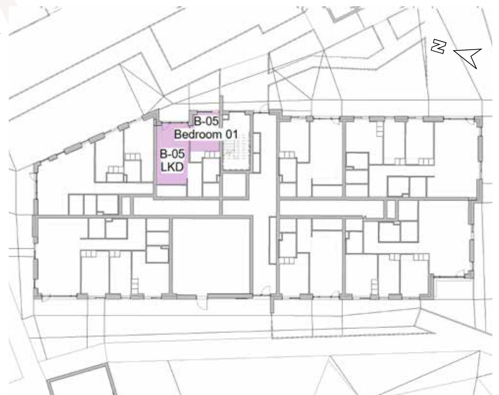
Figure 3.5: Below minimum recommendations for SE unit in Apartment Block B (Ground Floor), highlighting a recessed, self-obstructing design.
