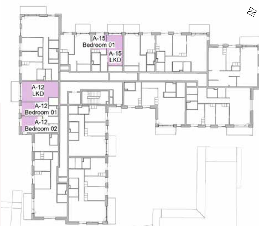
Figure 3.4: Below minimum recommendations for SE units in Apartment Block A (First Floor), highlighting a north-facing unit and a unit obstructed by balconies.
